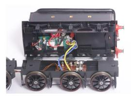
The completed radio control installation includes two wires from the tender to the loco. PVC is difficult to paint so I chose brown insulation to represent the grime found on the pipes near here on the prototype.
