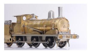
My completed Y14 loco has a new smokebox door, buffers, lubricator and cab roof, and a revised reverser reach rod. The rest of the model is straight from the Connoisseur kit.
