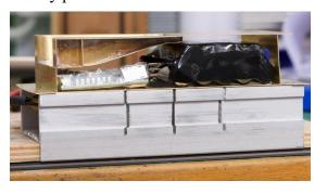
The most important design decision for the radio equipment is the style of the battery pack. I have used nine AAA size NiMh (rechargeable) cells arranged across the width of the tender. An odd number of cells will pack together sufficiently tightly to fit into the vertical space inside the body of the tender.
