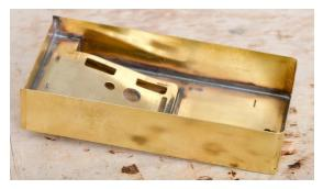
I cut three slots in the floor of the coal space to help the radio communications to work.
