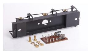
This created a tray-like space to hold a tag board with a fuse. The fuse is probably a
