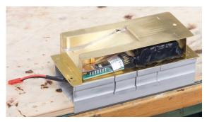
I built the tender body working from the top down, which is the opposite direction to that suggested in the instructions for the kit. I began by modifying the sides and floor of the coal space to make room for the two circuit boards to go underneath.
