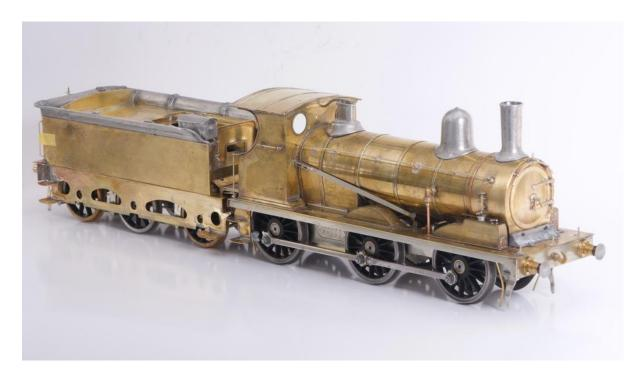
These notes describe how I fitted radio control into my model of a Great Eastern Railway class Y14. The loco and its tender are based on the Connoisseur Models kit for a LNER J15, with some alternative and extra parts.
