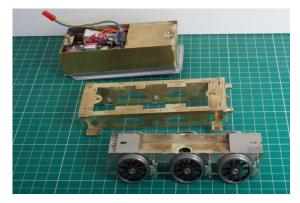
Construction then continued with the selfcontained footplate assembly and the chassis assembly.
