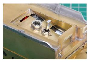
The charging socket and the toggle switch are easy to reach without lifting the model off the track.
