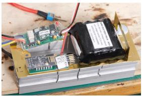
Here is a mock-up with the radio control parts arranged on the footplate of the tender. The rear bulkhead is resting loose here and I omitted it from the build to create more space for the battery pack. The parts are sitting on the mitre block to give me some space to hide the wires from the battery pack.
