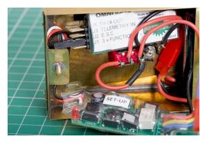
The wiring harnesses from Fosworks turned out to be too bulky to fit. I cut then down and added to new wiring to get everything to fit in.
