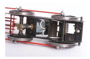
The pins on the Molex connector pass into a piece of stripboard on the other side of the frame spacer. I turned down the middle of the rear axle to make a clearance in front of the stripboard, and this was the only unplanned structural alteration needed during the build.
